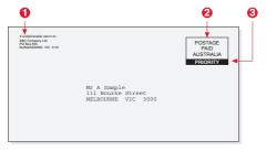
Clean Mail articles have to be suitable for Australia Post's automatic address reading equipment, so there are some mandatory correct addressing conditions, including font sizes and styles, and "clear zones" without any printing around the address area and on the back of the article.
